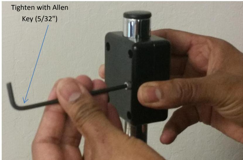
Install and tighten the remaining mounting (2ea) and clamp screws (1ea).
